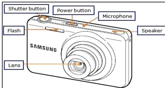
Fig. 1.4: Front and rear view of digital Camera and functions of various parts/buttons
