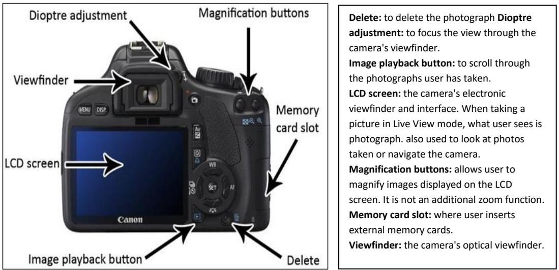
**Delete:** to delete the photograph **Dioptr adjustment:** to focus the view through the camera's viewfinder.
