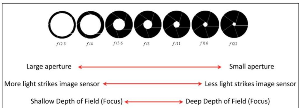
Fig. 1.7: Aperture Scale showing results of various settings
