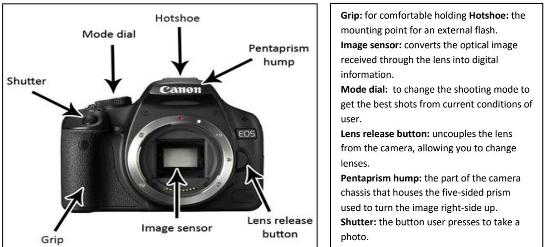
**Grip:** for comfortable holding **Hotshoe:** the mounting point for an external flash.
